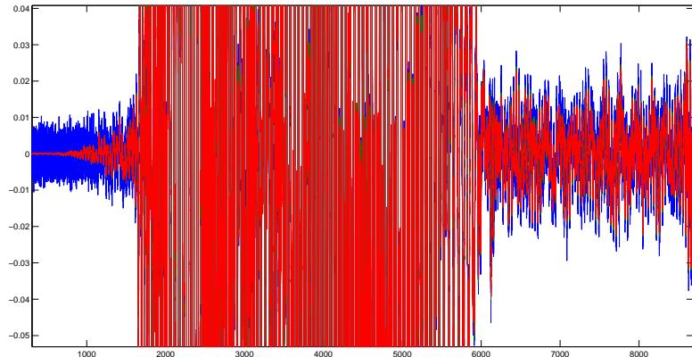
Figure 4: The same section of audio signal from Figure 3, but with a compression ratio of 2 to 1. Quantization errors are still spread throughout this signal, but there are less of them due to the lower compression ratio.
