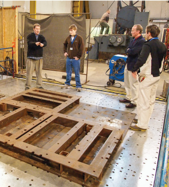
Engineer Matt Dolan (above, l.) explains how tested units are bolted to fixtures atop the aluminum vibration table.
