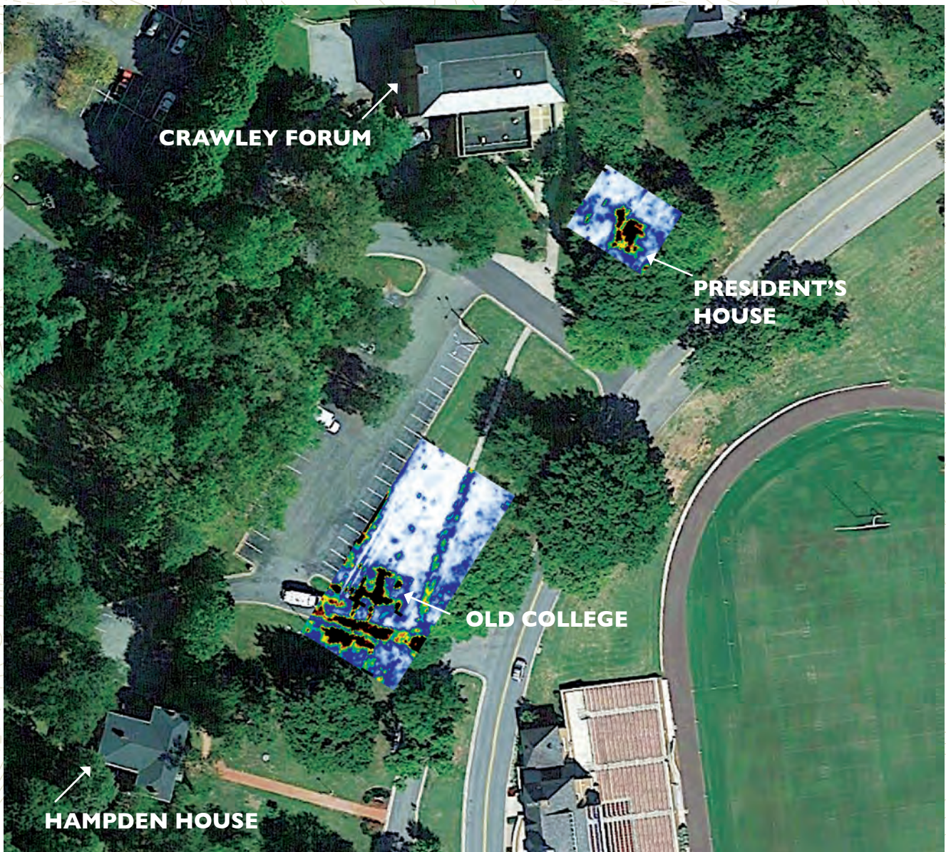
GPS Images show Old College remains at a depth of 60-70 cm and the President's House remains at a depth of 100-110 cm.
