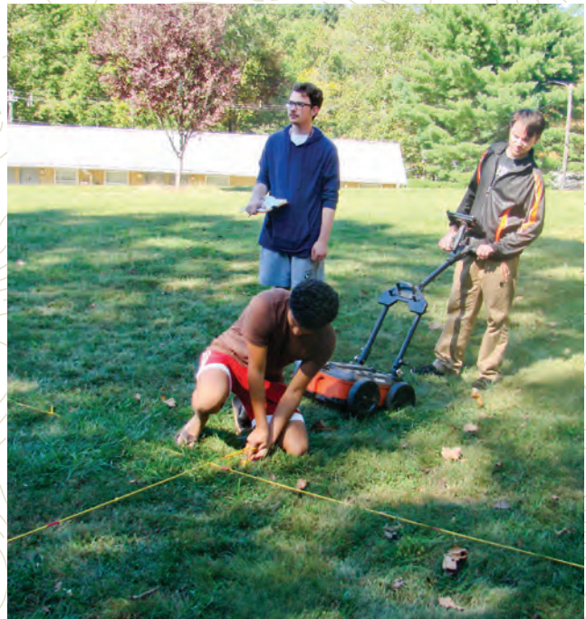
Thomas Alvarado '21 (kneeling), Jonah Popp '21 (l), and Ryan Gale '18 (R) establish survey lines and operate the GPR.
